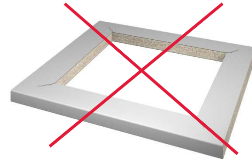
Incorrect practice – sharp edged corners
