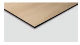
EGGER Compact Laminates Flammex CE are flame-retardant compact laminates according to EN 438-4, respectively EN 438-8 with a black core. They have a multilayer structure and consist of melamine resin impregnated decorative paper as surface layer and a fibrous and with curable resins impregnated core layer.
