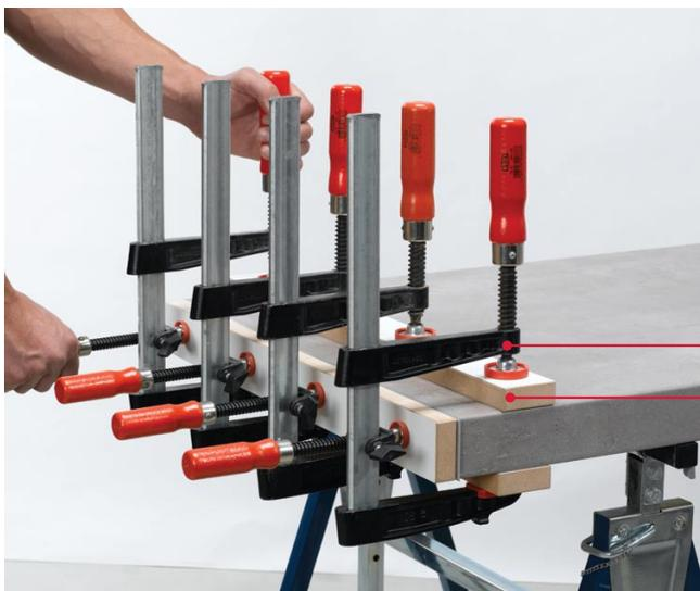
Conventional method of clamping should be used with spacing pieces and edge screw clamps
